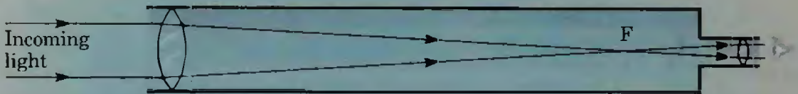
How a refractor works
